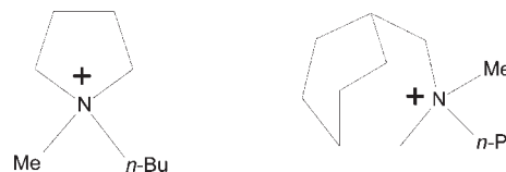
Figure 1. Structures of the N -butyl- N -methylpyrrolidinium and the N -methyl- N -propyl-3-azabicyclo[3.2.2]nonaneium cations.
